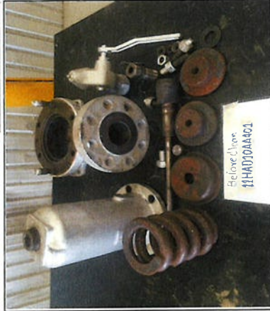
Valve disassembled
