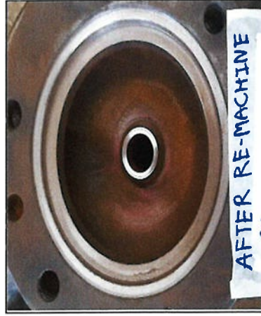
After Re-machine Nozzle (Seat)
