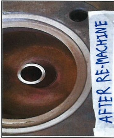
After Re-machine Nozzle (Seat)
