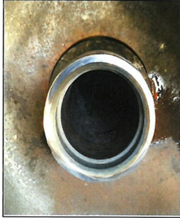
After Re-machine Nozzle (Seat)
