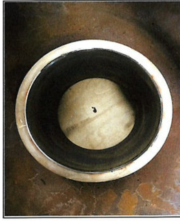
After Re-machine Nozzle (Seat)
