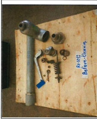
Valve disassembled & Before cleaning
