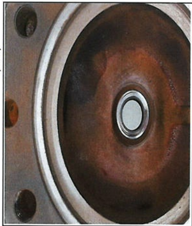
After Re-machine Nozzle (Seat)
