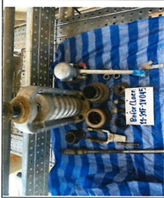
Valve disassembled & Before cleaning
