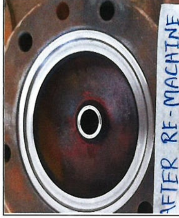
After Re-machine Nozzle (Seat)
