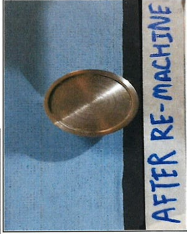
After Re-machine Disc
