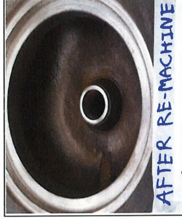
After Re-machine Nozzle (Seat)
